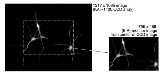
Figure 3. Monitor Display of CCD Image Center Area
